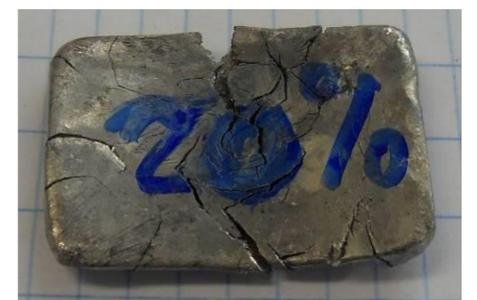
*Solder alloy MT-100640 (In<sub>57</sub>Sn<sub>17</sub>Bi<sub>26</sub>) (a) SEM picture of microstructure at enlargement 1000x (b) alloy cold rolled until cracked (20% thickness reduction).*
