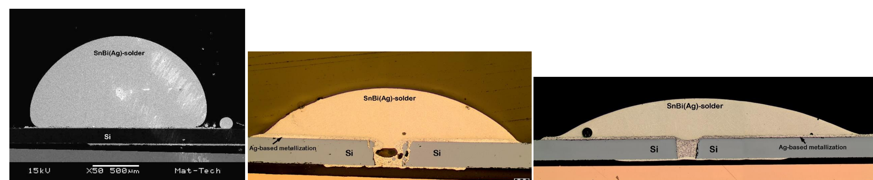
Fig. 2: Cross-sectional view of the “sessile drop” of the Bi57Sn42Ag1 solder after reflow on Ag-based metallization in the test samples received from (left) supplier A (Secondary Electron Image); (center) supplier B (bright-field optical image) and (right) supplier C (bright-field optical image).
